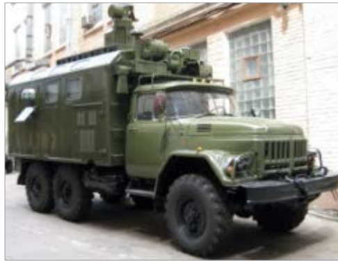
Figure 2 - Optical-electronic countermeasure complex “Kashtan-3(M)”
