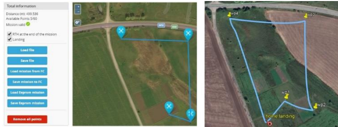
Figure 12 The comparison of the quadcopter planned and real flight by points.
